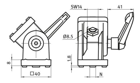
For movable or rigid profile connections at any angle from 0° to 180°.
