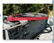
Solution On upgrading to PowerTwist Plus V-Belts, the maintenance team now carries boxes of the red belt 24/7. Drives are now serviced quickly without wasting time returning to the belt crib to pick up specific belt sizes. Stock was reduced to just a few boxes of 3L, A/13 and B/17 sections.
