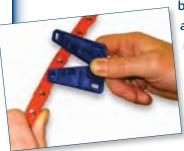
belt off, take out a link and roll it back on — no need to move any drive components.
