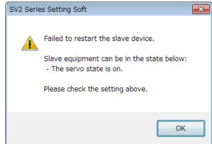
**Reference** The software reset is used for the slave machine restart from the SV2 series setting software. If a warning appears, the restart may have failed, so check the reason.
