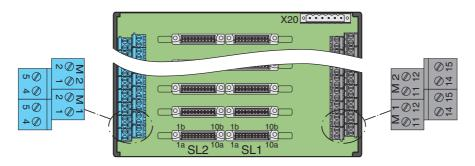
Insert the isolated barrier on the Termination Board. This closes the signal circuit between field side and control side. Connect field devices and controller to the terminals or connecting plugs of the Termination Board. For pin assignment between terminals, connecting plugs and connectors SL1/SL2, see drawing "Connection diagram" or the corresponding pin-out table on www.pepperl-fuchs.com.
