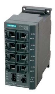
SCALANCE X208, managed IE switch, 8x 10/100 Mbit/s RJ45 ports, LED diagnostics, error-signaling contact with set button, redundant power supply, PROFINET IO device, network management, Redundancy Manager integrated, incl. electron. manual on CD-ROM, C-plug optional
